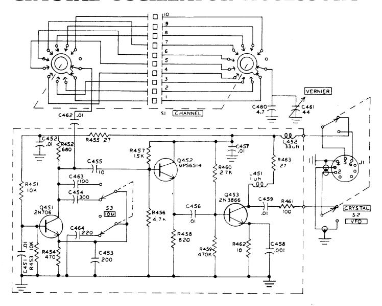
The Model 10XB oscillator provides for added versatility with the Atlas transceivers by crystal controlling the operating frequency. Vernier frequency adjustment is provided and a switch selects either crystal or VFO control. A ten position switch allows selection of up to ten crystal frequencies.
